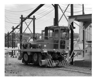
In addition to the diesel switchers mentioned in the text, Blue Ridge uses this Rail King switcher.
